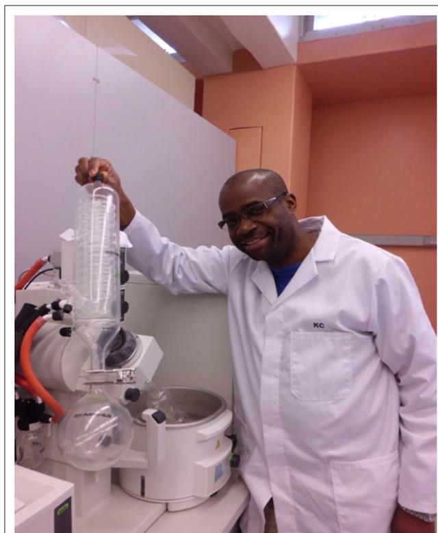
Kelly Chibale with his rotary evaporator, which is used to remove solvents from organic solvent solutions and to isolate the molecule of interest – in this case, the drug’s lead molecule (photo: Jenny Leonard).
