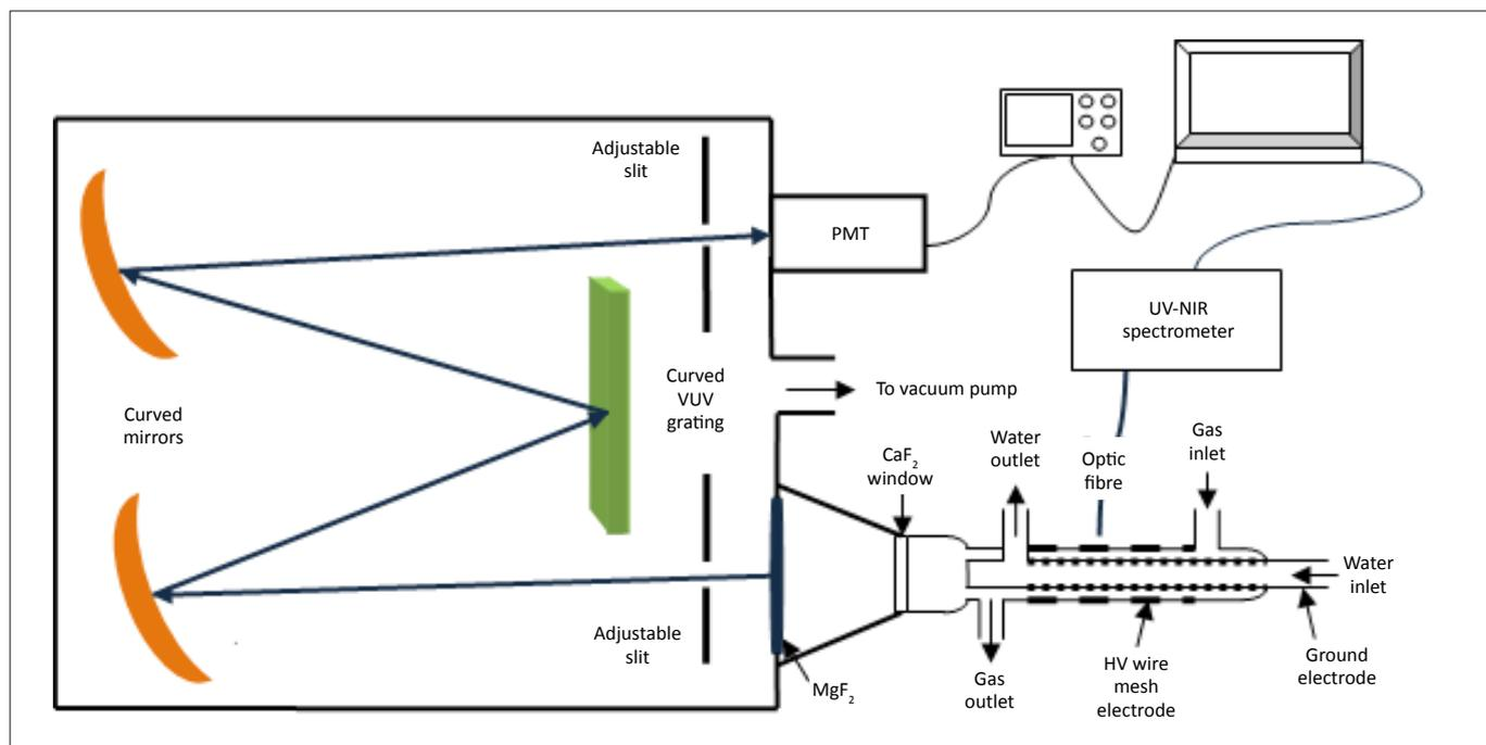
PMT, photomultiplier tube; UV-NIR, ultraviolet-near infrared; VUV, vacuum ultraviolet; HV, high voltage.
