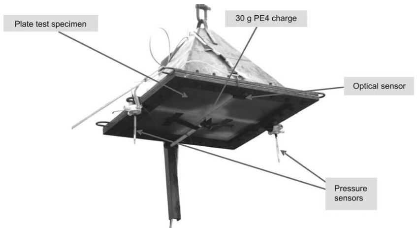
Fig. 6. The position of the optical sensor, relative to the pressure sensors, for Events 4 and 5.
