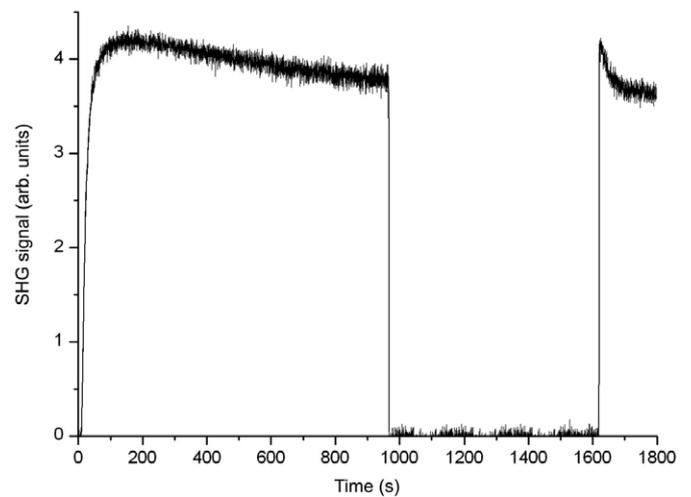
Fig. 3. Interrupted time-dependent SHG signal from Si/SiO<sub>2</sub>. The sample was irradiated for about 16 min after which the beam was interrupted for about 11 min before irradiation continued for about another 3 min.
