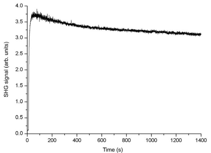
Fig. 2. Time-dependent SHG signal obtained from Si/SiO<sub>2</sub> by irradiating a single spot on the sample for about 23 min.
