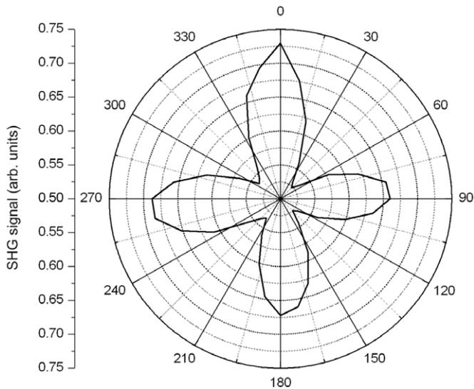
Fig. 4. Polar plot showing the rotational anisotropy pattern of the equilibrium EFISH signal obtained from Si/SiO<sub>2</sub>.
