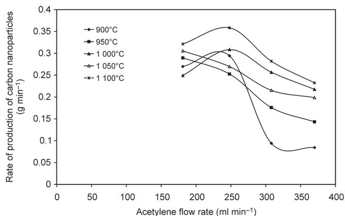
Fig. 6. Effect of pyrolysis temperature on the rate of production of carbon nanomaterials at different acetylene flow rates.
