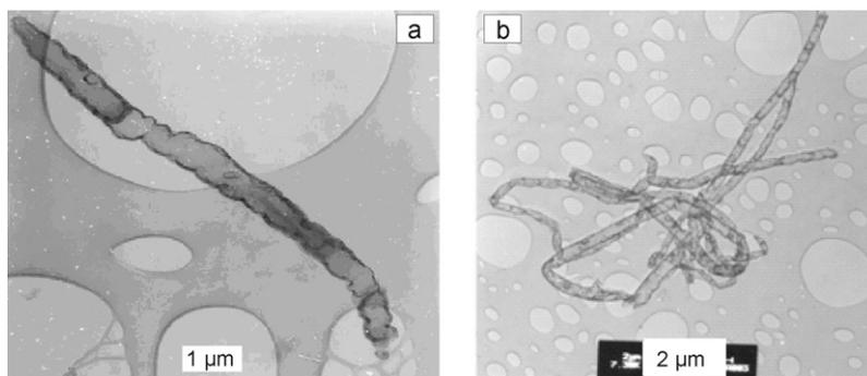
Fig. 2. High-resolution transmission electron microscopy images of (a) as-synthesised SWCNT obtained at 10% ferrocene and 1 100°C and (b) purified SWCNT obtained at 5% ferrocene and 1 000°C.
