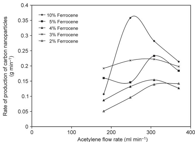
Fig. 5. Effect of ferrocene concentration on the rate of production of carbon nanomaterials at different acetylene flow rates.
