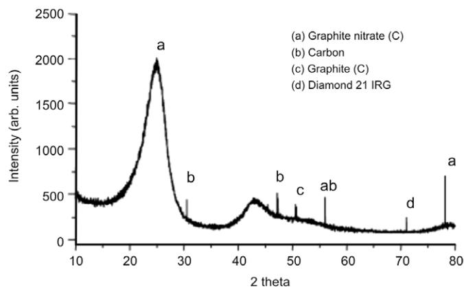
Fig. 8. X-ray diffraction analysis of a sample produced at 10% ferrocene, 1 100°C and a hydrogen flow rate of 181 ml min<sup>-1</sup>, confirming traces of diamond films.
