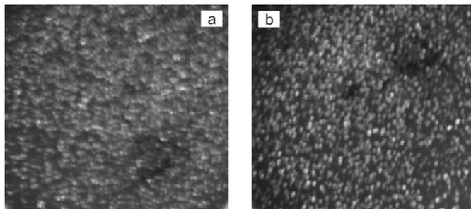
Fig. 7. Photographic images (EuroTEK 10 Megapixels) of diamond films obtained at (a) 10% ferrocene, 1 000°C and a hydrogen flow rate of 118 ml min<sup>-1</sup>, and (b) 10% ferrocene, 1 100°C and a hydrogen flow rate of 181 ml min<sup>-1</sup>.
