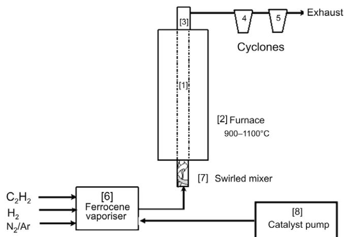
Fig. 1. Schematic of the swirled floating catalyst chemical vapour deposition reactor.<sup>33</sup>
