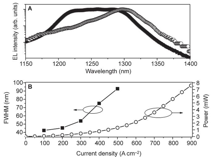
**Fig. 4.** Comparison of electroluminescence (EL) from a 3 × 2 superluminescent diode (solid) and a standard dot-in-a-well (open) for 500 mA (A). Power and full width at half maximum (FWHM) as a function of continuous current are also shown for the 3 × 2 device (B).
