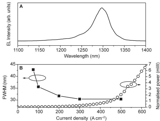
**Fig. 3.** Electroluminescence (EL) from a 6 mm dot-in-a-well superluminescent diode at room temperature and 100 A cm<sup>-2</sup> (A). Power and full width at half maximum (FWHM) as a function of continuous current are also shown for this device (B).
