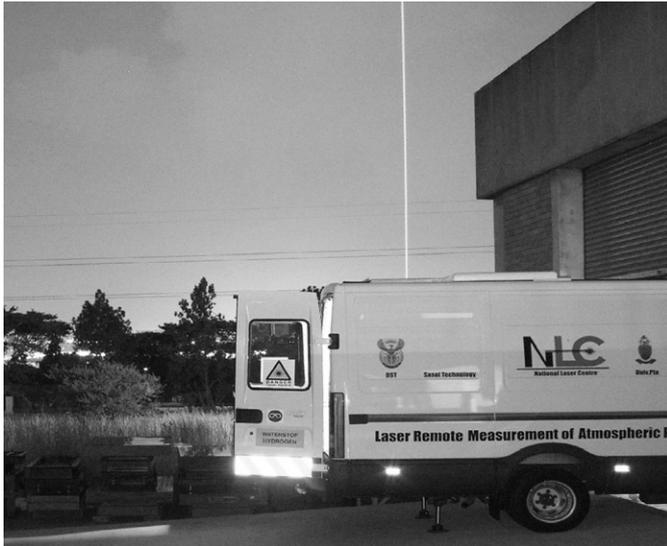
Fig. 1. The CSIR-NLC mobile LIDAR system.
