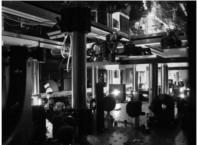
**Fig. 2.** View of the amplification stages of the JETI 10-TW Ti:sapphire laser system at the University of Jena, Germany. The illumination is scattered light of the Nd:YAG pump lasers, the bright spot in the centre of the picture is a fluorescing Ti:sapphire crystal in one of the multi-pass amplification stages.
