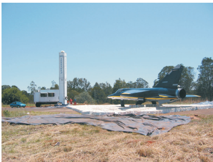
Fig. C. The Mirage F1 airframe on the measurement platform. The antenna tower and laboratory can be seen in the background.
