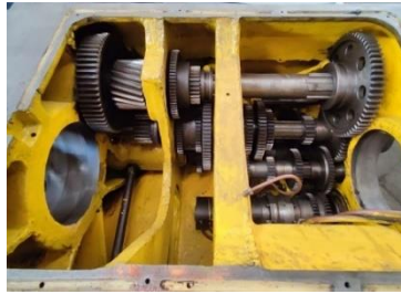
Figure 2: Internal diagram of remanufactured spindle box
