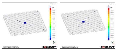
Figure 19: Solidification of product (left side conformal; right side conventional) (see online version for colour)
