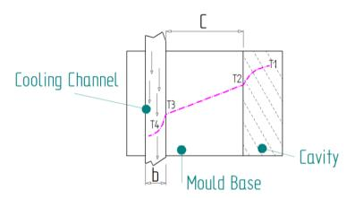
Figure 2: Cooling channel design parameters
