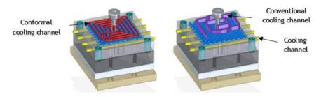
Figure 18: Conformal and conventional cooling channels
