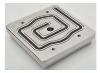
Figure 4: Cooling channels manufactured using conventional machining methods
