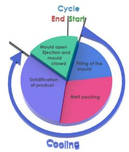
Figure 1: Injection moulding cycle
