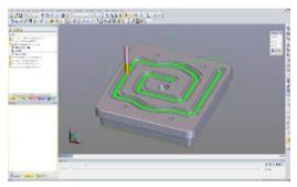
Figure 10: NC toolpaths programmed using EdgeCam 2014 R1
