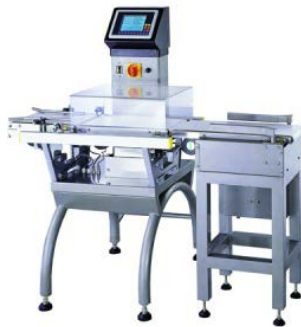
Figure 2.7: Automated external check-weighing module
