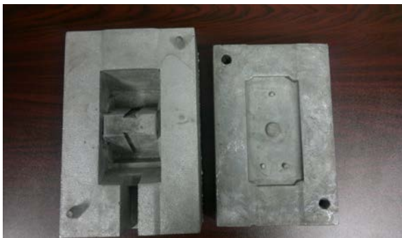
Figure 2: (a) CAD of the lower part of the die; (b) DCP mould; (c) RCT die - cast before finishing operations
