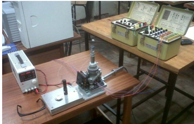
Figure 3: Experimental setup for residual stress measurements
