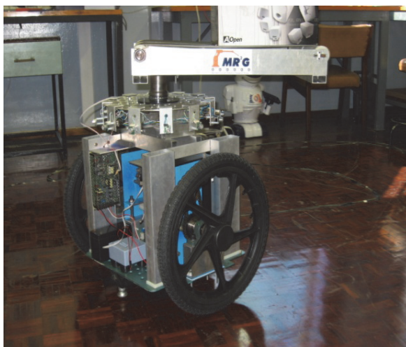
Figure 4: AGV for distributed process integration
