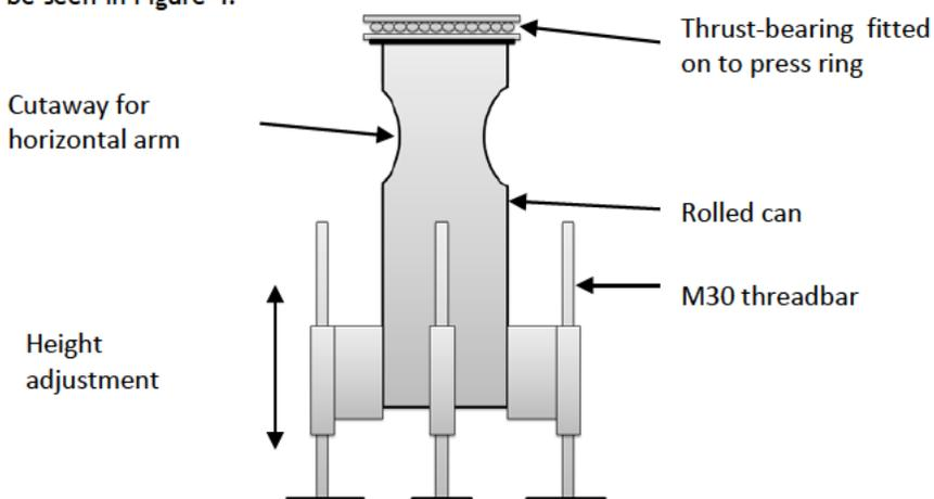
Figure 4: The skeletal structure of the tool changer (adapted from [6])
