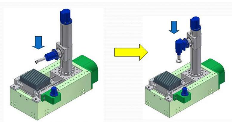
Figure 2: Using different modules to vary a machine's functionality [3]
