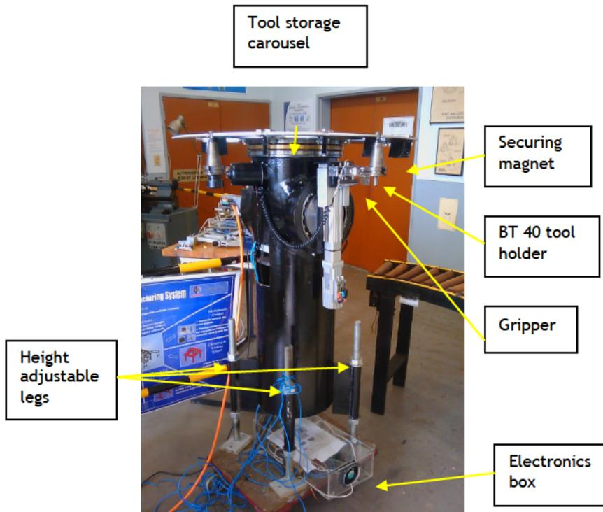
Figure 6: The completed tool changer (adapted from [10])
