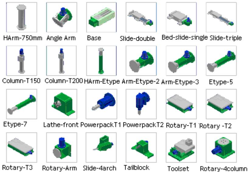
Figure 1: An example of a library of modules for modular reconfigurable machines (adapted from [3])
