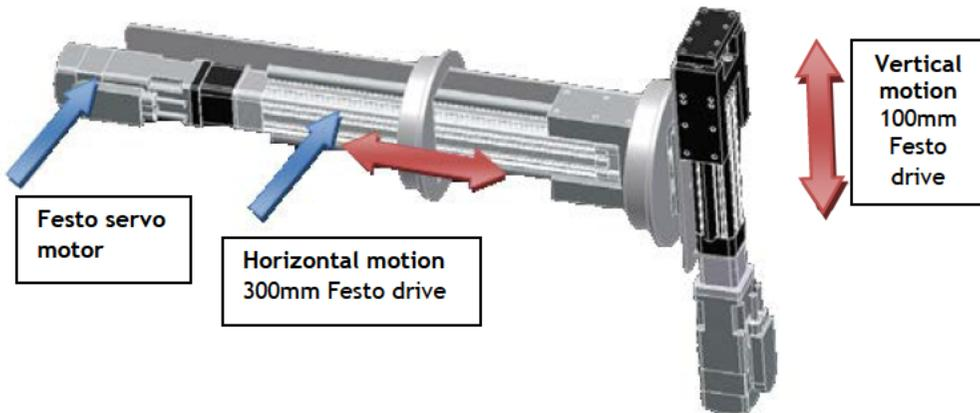
Figure 5: Spindle drive configuration (adapted from [6])
