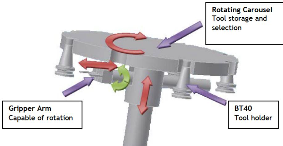
Figure 3: Tool-changing module concept [10]
