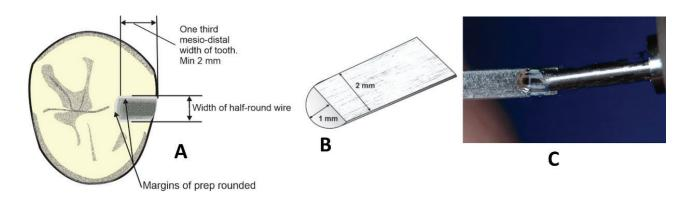
Figure 6A: The dimensions of a posterior rest seat for a half-round wire rest. B: the recommended size of the half-round wire. C: choose a bur slightly smaller than the width of the wire, ie a .018 round bur.
