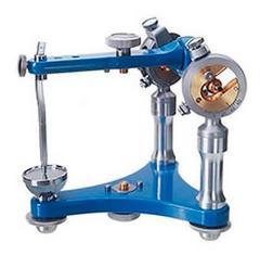
Fig. 6. A non-arcon articulator: the 'condyle is on the upper member and the 'fossa' on the lower member.
