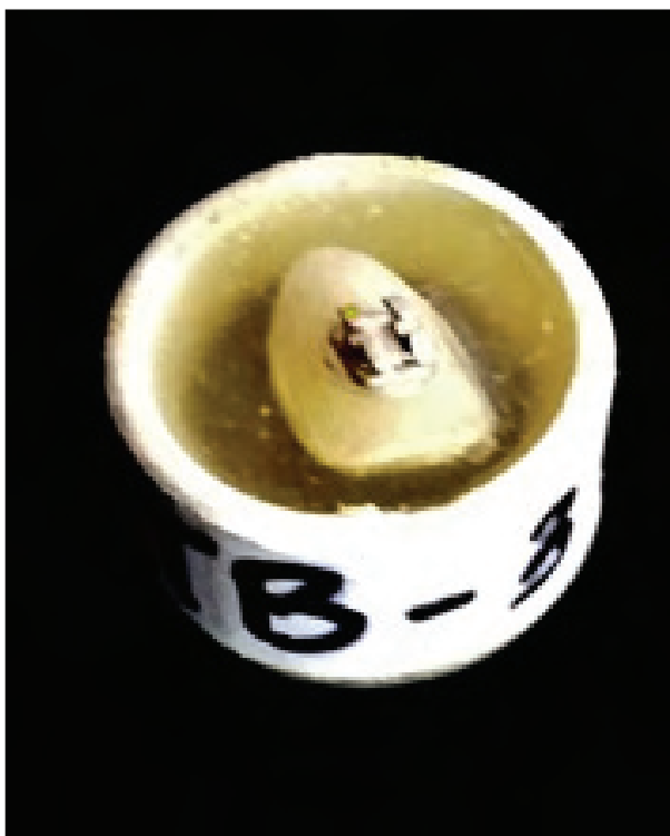
Figure 2: Crown embedded and bonded with a metal bracket. Labelled according to particular groups.
