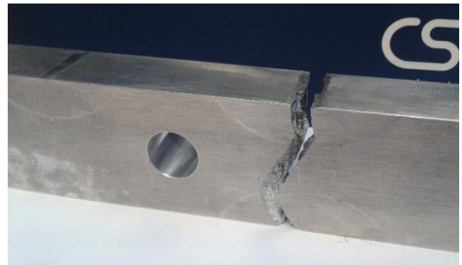
Figure 10 Photograph of fractured specimen (first mod.)
