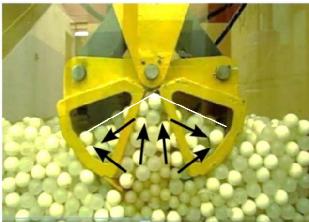
Figure 8: Motion of plastic spheres into interior of buckets
