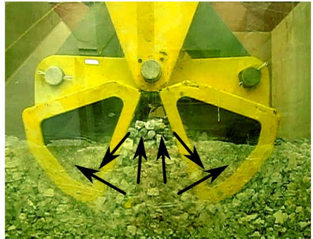
Figure 10: Motion of stone aggregate into interior of buckets
