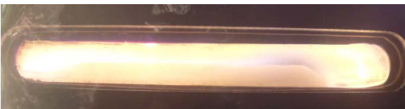
Figure 17: Combustion of Sasolwax 0907 with nitrous oxide
