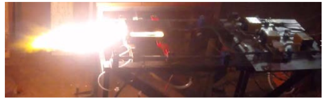
Figure 18: Still image captured from video footage of hot fire test
