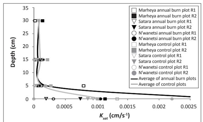
$K_{sat}$  saturated soil conductivities; R1, Replicate 1; R2, Replicate 2.
