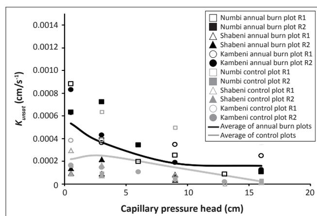
$K_{unsat}$  unsaturated soil conductivities; R1, Replicate 1; R2, Replicate 2.
