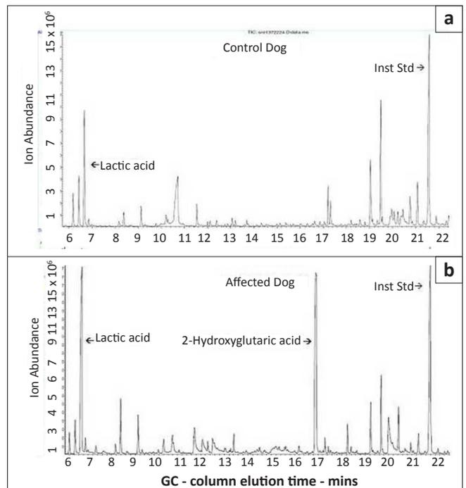
X-axis, gas chromatography column compound elution times; Y-axis, Fragment ion abundance in arbitrary units
