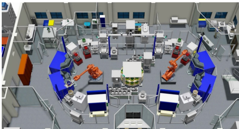
Figure 7—Robotic automated facility for sample preparation and analysis for chemical, PSD, and moisture
