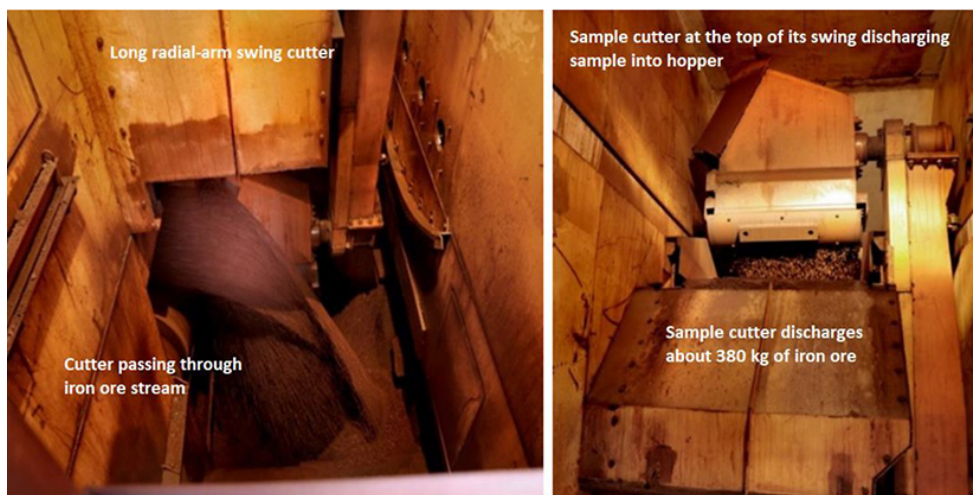
Figure 5—Swing-arm cross-stream sampler and discharge of 370 kg iron ore sample into hopper
