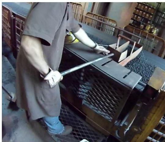
Figure 1—Stop-belt sampling on the waste conveyor
