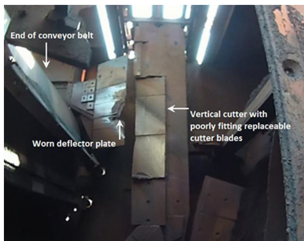
Figure 2—Poorly designed cross-stream sampler at the end of a conveyor belt
