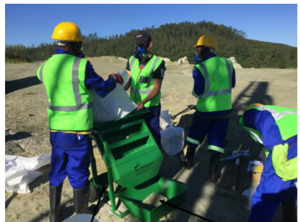
Figure 6—Sampling team preparing samples with riffle splitter
