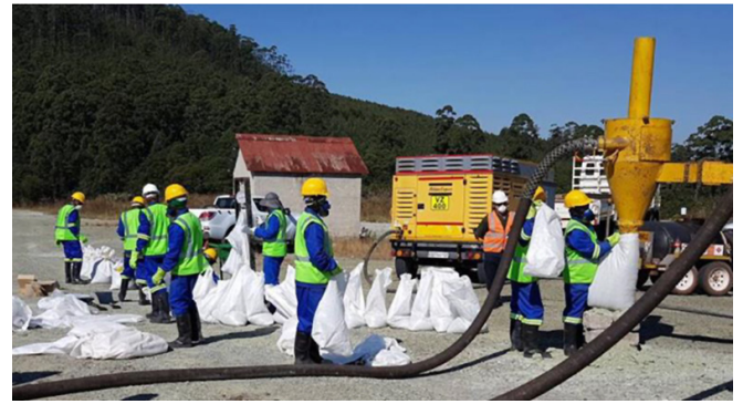
Figure 5—Sampling site in the Havelock exploration programme: four samplers collected the tailings material from the cyclone of the air core drill rig
