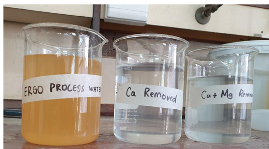
Figure 13—Comparison of process water after softening treatment
