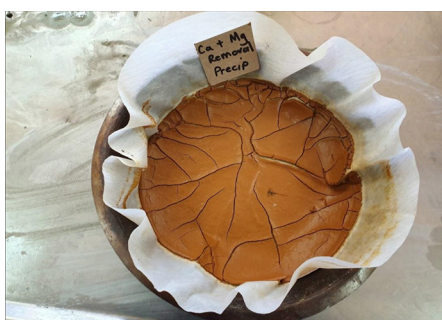
Figure 12—Filtered precipitate for lime plus soda ash softening at ambient conditions
