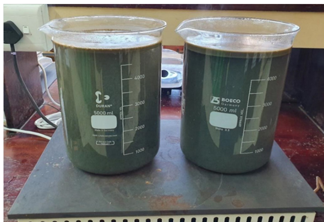
Figure 10—Two 5 litre glass beakers of process water treated with unslaked lime (CaO)
