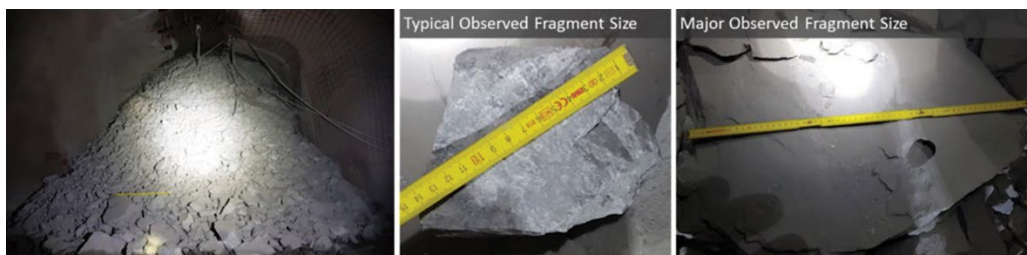
Figure 16—Post-blast results (after Paredes and Rodriguez, 2018)
