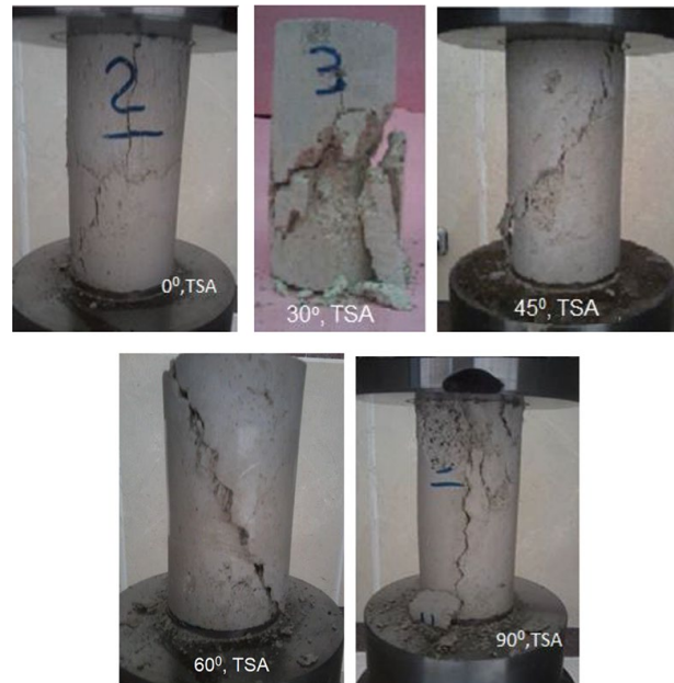
Figure 5—Mode of failure of five specimens with TSA discontinuities at orientation angles of 0, 30, 45, 60, and 90 degrees under uniaxial loading
