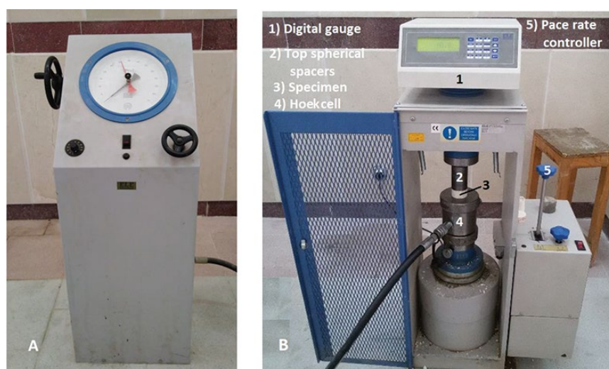
Figure 4—ELE triaxial compression test apparatus: (A) Confining pressure, (B) adjustment of specimen and spherical spacers inside the triaxial cell and between the platens of the testing machine
