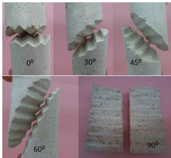
Figure 2—One series of specimens with tooth-shaped asperity discontinuities with different orientation angles
