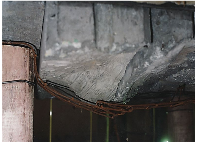
Figure 5— Containment, by a steel strap, of discontinuous, displaced hangingwall in a simulated stope subjected to a drop weight impact
