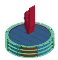
Figure 7-Complete numerical model of the rope platform
