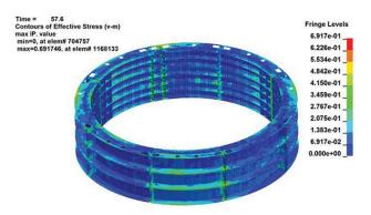
Figure 15—View of the maximum tensions applied to the ring with the reduced steel sheet thickness, unit (GPa)
