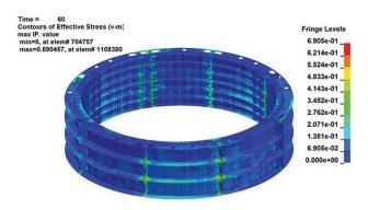
Figure 14—View of the maximum tensions applied to the ring with the initial steel sheet thickness, unit (GPa)
