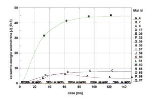
Figure 13—Internal energy of individual model segments, A – ropes, B – boards, C – T-bars, D-Q – ring segments
