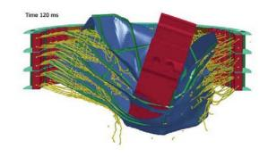
Figure 11—Platform cross-section at the point when the impacting cover stopped (120 ms)
