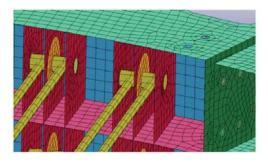
Figure 8-Connection of the rope net to the ring
