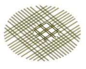
Figure 6-Discretization of the rope net
