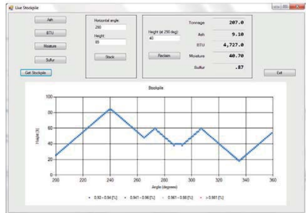
Figure 16—Stockpile's shape after reclaiming to 12 m (40 ft)
