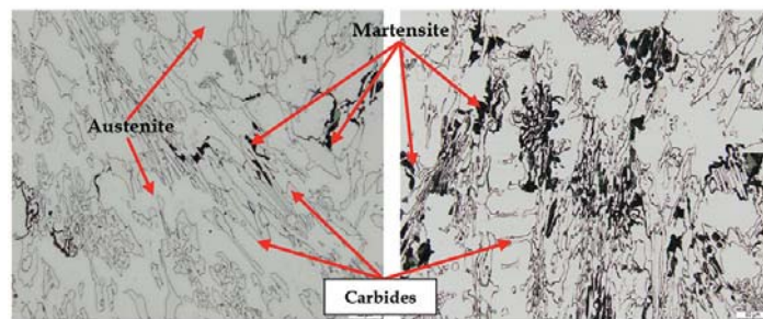
Figure 3—Microstructures of HCWCI with 0.1–0.4% and 0.4–0.6%Nb showing the presence of martensite at the carbide interface
