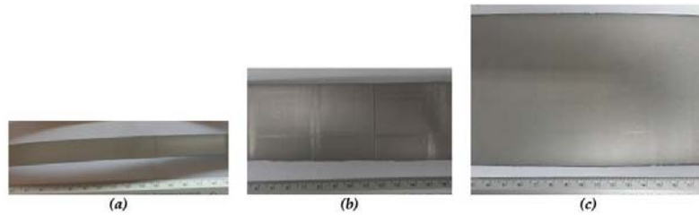
Figure 7—Photographs of Ti HDH 100 mesh strips rolled at 0.3 mm roll gap and (a) 20 mm, (b) 50 mm and (c) 100 mm set widths
