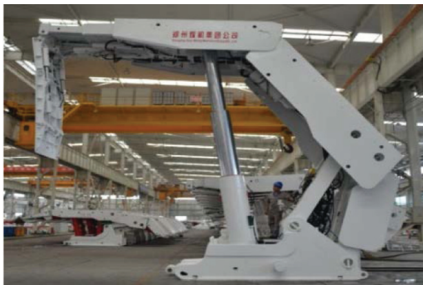
Figure 2 – Type ZY15000/33/72D shield used at Wangzhuang
