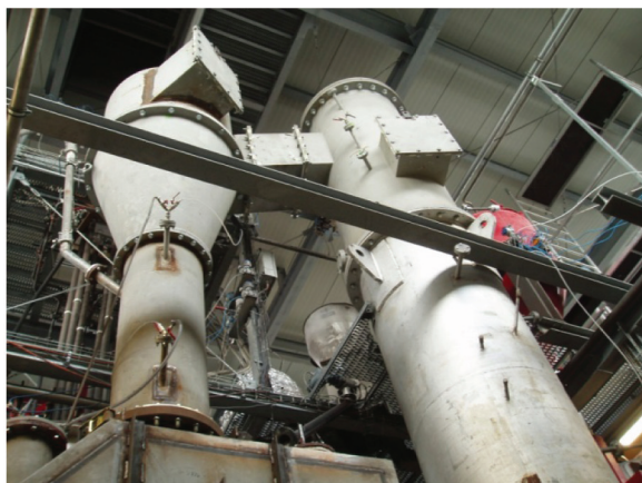
Figure 8 – State-of-the-art HTW™ pilot plant (0.5 MW thermal input), located at the Technical University of Darmstadt, Germany
