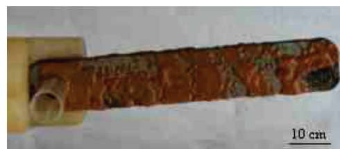
Figure 1—A typical corrosion coupon after exposure
