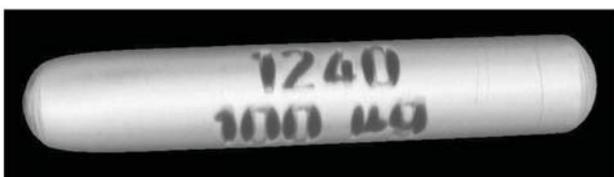
Figure 11 –  $\mu$ XCT of a Ra isotopic source ampule (Hoffman, 2012)
