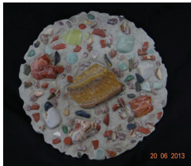
Figure 7 – Brecciated jasper, marble, jasper and tiger's eye cemented at Mintek
