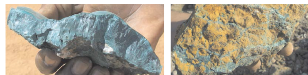
Figure 3—Malachite (left) and chrysocolla (right) ores
