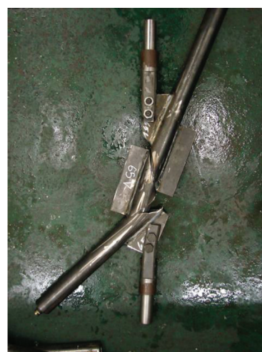
Figure 9—A test jig with 65° installation angle and vertical failure plane, where failure has occurred on the test jig itself
