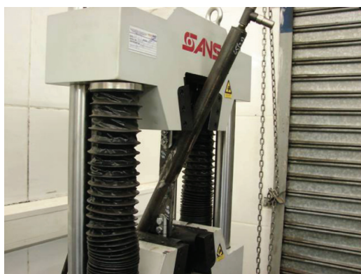
Figure 7—Test set-up for a tendon installed at 60° with a horizontal failure plane
