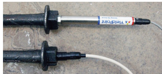
Figure 4—Instrumented roofbolt with an extended-length head (top) and shallow head (bottom) (Kostecki, 2013)
