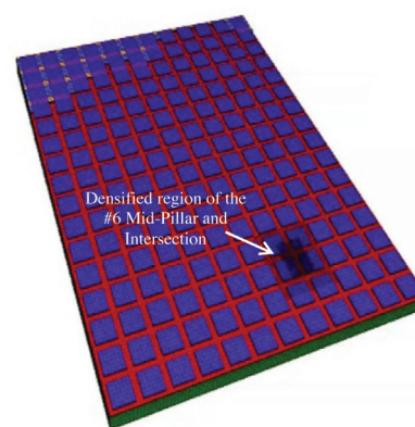
Figure 22—The global grid showing the excavation sequence and the densified region of the FGPR bolts
