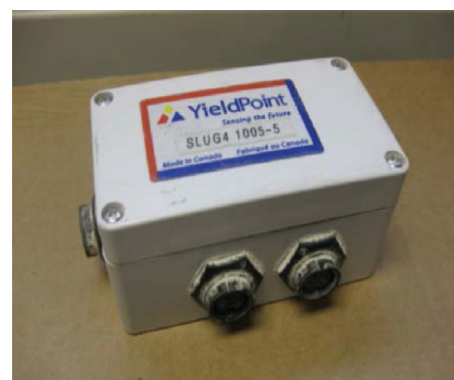
Figure 6—d4 logger data-log box by YieldPoint Inc. (Kostecki, 2013)
