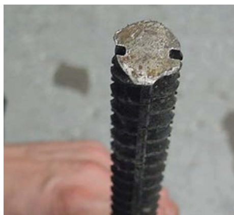
Figure 3—Slotted rebar for sensor placement (Kostecki, 2013)
