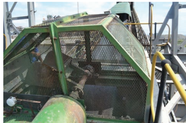
Figure 4—0.45 m cutter on 1.35 m belt for primary sample. The cutter sweeps an increment into the impact crushers
