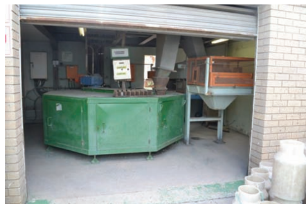
Figure 5—Indexed carousel used to collect samples crushed to 8 mm
