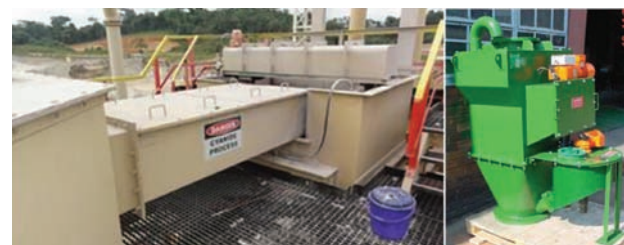
Figure 14—(a) Cross-stream launder sampler (left) and (b) a 2-in-1 sampler (right)
