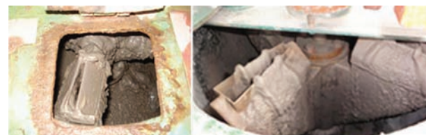
Figure 18—Collectors of Vezein-type samplers clogged by accumulated slurry material
