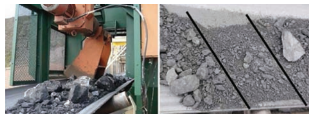
Figure 12—(a) Go-belt sampler in operation (left), and (b) material remaining on the belt after sampling (right)
