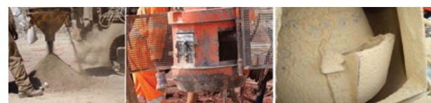
Figure 4—(a) Stationary cone splitter, which must be perfectly levelled before use (left), (b) rotating cone splitter (middle), and (c) stationary or rotating cone splitter with slots in the cone (right)
