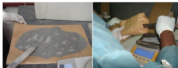
Figure 20—Examples of aliquot selection in a laboratory. (a) Dip sampling method and (b) using a spatula along the full length of the packet
