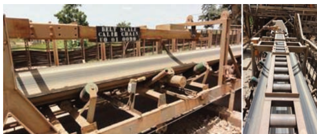
Figure 10—Calibration of the plant feed weightometer using (a) the zero test, and (b) a static weight test
