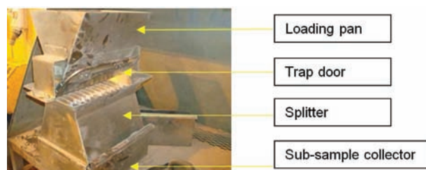
Figure 6—Riffle splitter with a manual sample dispenser correctly placed along the mid-line of the riffles below it
