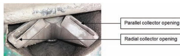
Figure 17—Radial (correct) and parallel (incorrect) collectors of a Vezein-type sampler
