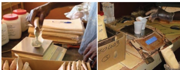
Figure 21 – Examples of incorrect methods of aliquot selection in a laboratory by (a) pouring the pulverized rock from the packet and (b) scooping the powder from the packet with a spoon
