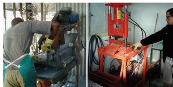
Figure 1 – Sub-sampling by means of a diamond saw (left) and a guillotine (right)
