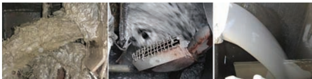
Figure 16—Examples of cross-stream slurry sampler collectors
