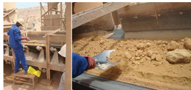
Figure 11—Broken ore on a moving conveyor is grab-sampled by means of a spade
