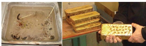
Figure 19—(a) Bullion dip samples (left) and (b) a drilled bullion bar (right)
