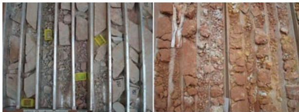
Figure 2—Borehole core from carbonaceous reef (left) and saprolite(right)
