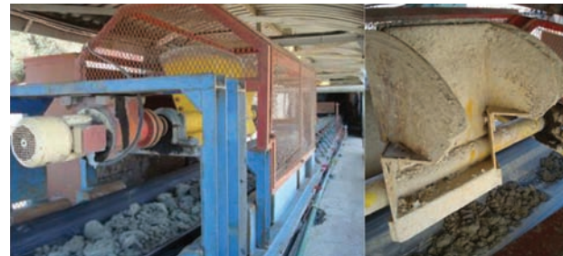
Figure 8—A go-belt sampler (left), and the sample collector (right)
