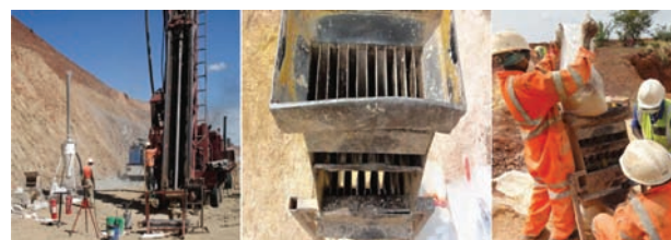
Figure 3—(a) Cyclone (left), (b) riffle splitter (middle), and (c) splitting process (right)
