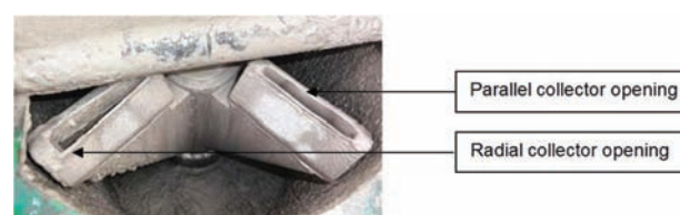
Figure 17—Radial (correct) and parallel (incorrect) collectors of a Vezin-type sampler
