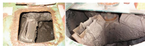
Figure 18—Collectors of Vezin-type samplers clogged by accumulated slurry material
