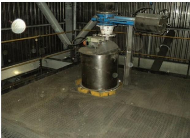
Figure 2—Primary Vezin sampler
