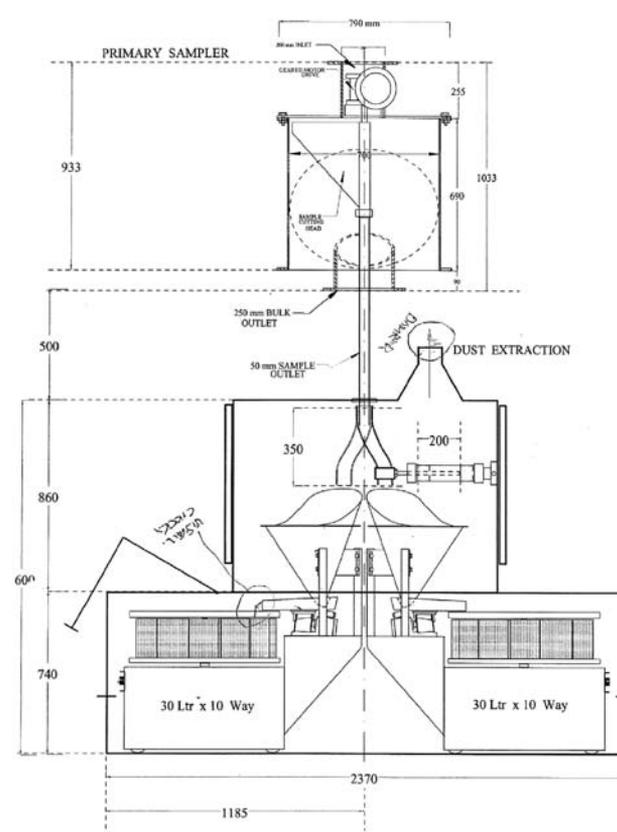
Figure 1—Schematic design of Vezin sampler and the two rotary splitters used to collect the interleaved increments from the Vezin
