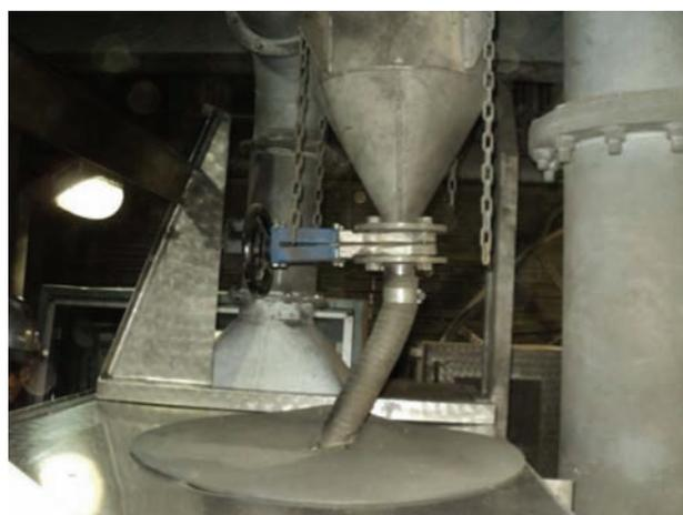
Figure 7—Intermediate hopper between primary Vezin and 10-way splitter hopper
