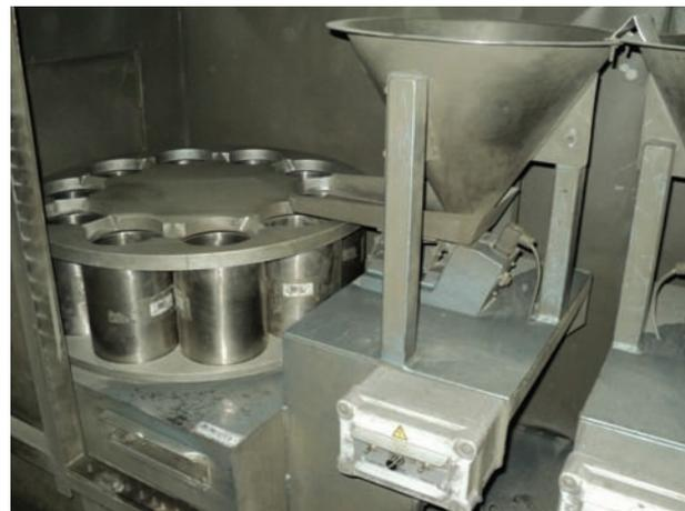
Figure 4—10-way splitter used for the sub-sampling of the interleaved samples
