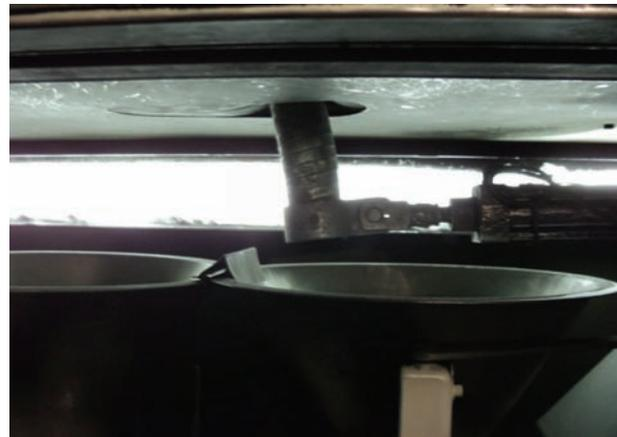
Figure 3—Oscillator to direct a flexible tube channelling the sample into the respective hoppers
