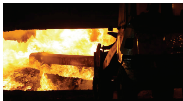
Figure 6 – Example of an open furnace used to produce SiMn being fed through a feed chute in the roof
