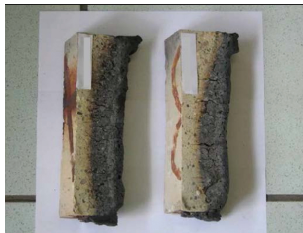
Figure 5—Sectioned rotary slag test samples
