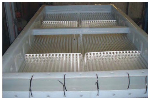
Figure 1—Condensing heat exchanger (gas/gas) with mechanically attached PFA lining (Courtesy Panergetic AG, Liechtenstein)
