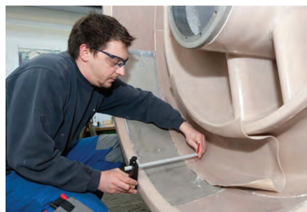
Figure 3—Fabrication of the bonded FEP lining for an industrial steel centrifuge. Thermo-formed liner segments are cut to shape before gluing them into the steel structure. (Angenstein AG, Switzerland)
