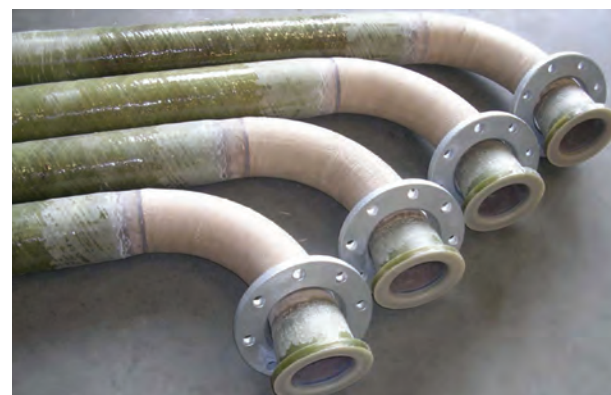
Figure 4—Prefabricated FRP-reinforced liner pipe sections. Straight liner pipe sections were reinforced using a filament winding machine. Liner pipe elbows (at this stage not yet FRP-reinforced) and flanges inserted by hot gas welding. Subsequently, the elbow section will be FRP-reinforced by hand lamination (courtesy PRP Plastic OY, Finland)
