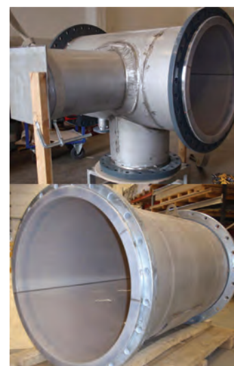
Figure 7—Blast spools for sulphuric acid-containing gas (courtesy PRP OY, Finland)
