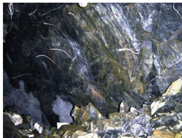
Figure 5—Rockbolts indicating upwards direction of ejection (photograph T.R. Stacey)
