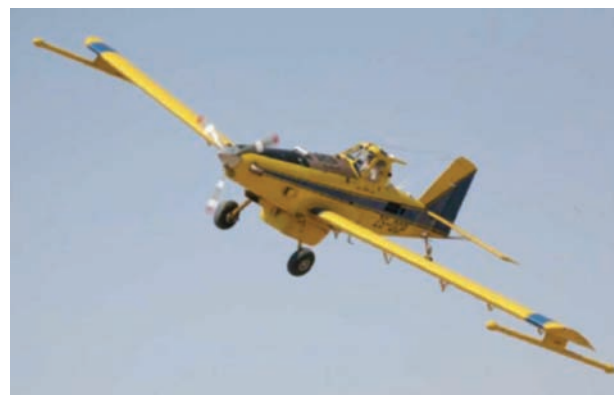
Figure 4—Air Tractor system used by Xcalibur Airborne Geophysics used for high-resolution aeromagnetic survey over the southern CKGR
